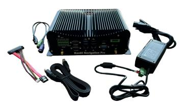
Kordil Fanless Industrial Mini PC, is a compact computer system designed to operate reliably in heavy industrial conditions and sensitive applications such as coastal surveys. Specifically engineered to seamlessly function in challenging industrial environments prone to extreme temperatures, water, dust, humidity, and vibrations, this system offers unparalleled reliability.
